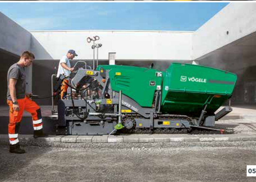
01 Large material hopper with a capacity of 5.8 t. 02 Traction drives in closed loops deliver both positive tracking when moving straight and precise steering. 03 Innovative, easy-to-operate ErgoBasic operating concept for simple handling.
